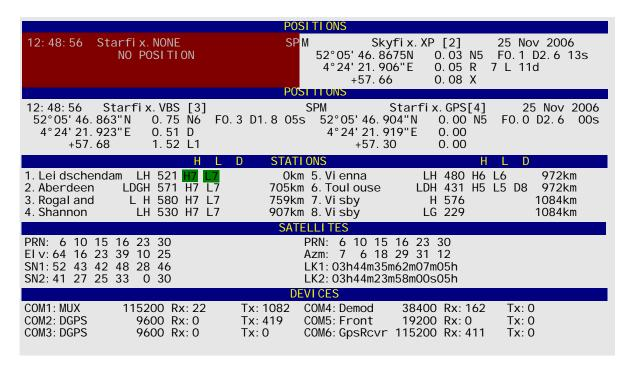
In this example all is going well, still the display for positioning is saying "No Position". This is due to the setting in the SPM menu which has set the display to "None", notice the text above also saying "Starfix-NONE". Change the setting back to HP, see section  $9.6.2 \text{ SPM Menu} \rightarrow \text{Positioning} \rightarrow \text{Position Views}$ .
