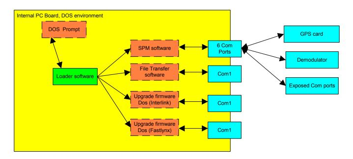
Figure 2 Software on the processing board
