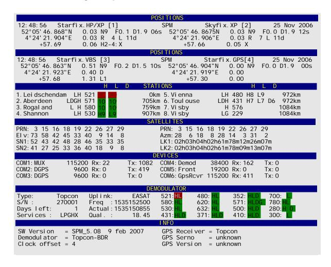
Station Leidschendam (521) is down for maintenance, as indicated by the red colour behind the station. If a station drops out for no clear reason, the following can be done.
