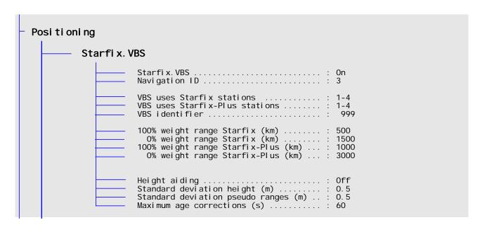
Starfix VBS is Fugro's Virtual Base Station solution. The solution uses the L1 (L) and/ or L2 (D). Read for more information section 5.4 Theory of the VBS Position Calculation.
