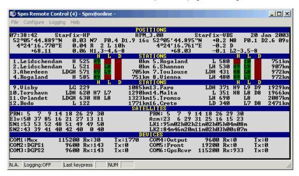
From here, the Starfix SPM unit can be configured, and addition device drivers started.
