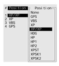
This determines which positions are shown on positions 1 to 4 in F1 - Positions Display.
