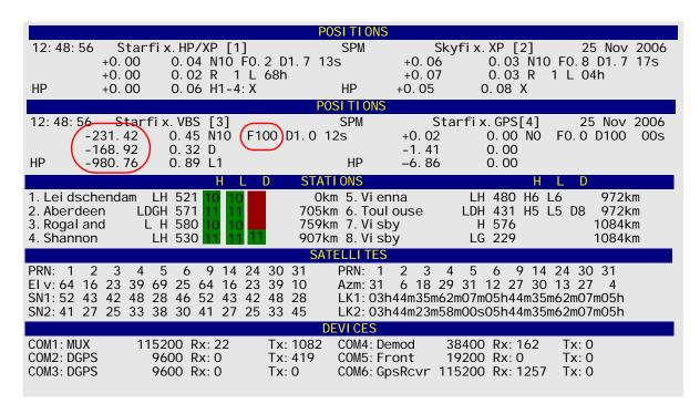
The VBS position is clearly wrong as indicated by the large Deltas. Also F-test result (F100) indicates that VBS position is not valid. When the F-test is this high, then the standard deviations are not realistic anymore.
