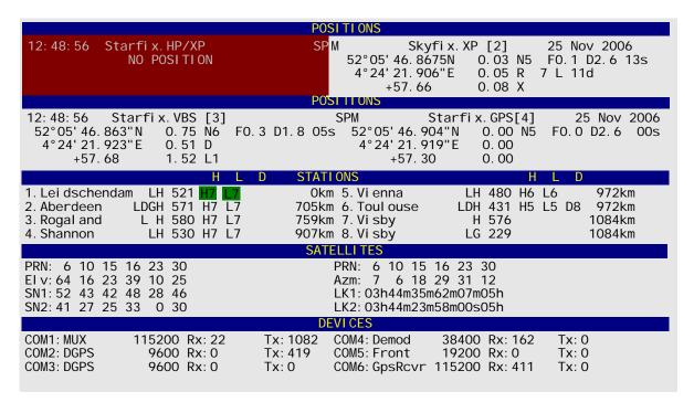
The text "No Position" indicates total failure of the calculation to work.
