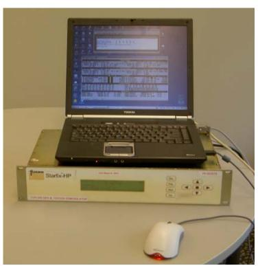
Connect a null modem cable between the HP Mobile Com1 and the computer.
