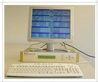
The keyboard and monitor are connected to the back panel of the HP Mobile.
