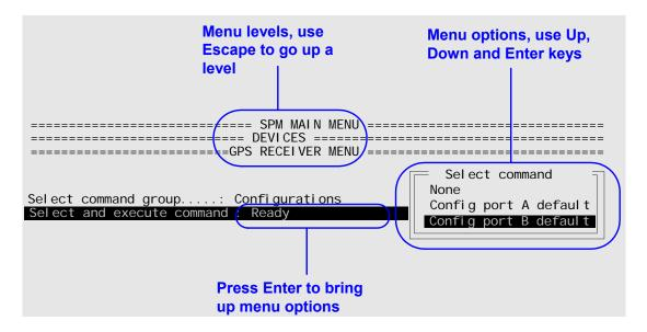
When operating the SPM through a keyboard, one can use the Enter, Escape and F1 to F6 keys and well as all the numbers and characters for typing. This is an advantage over the front panel operation.
