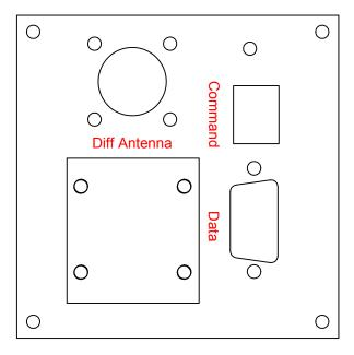
The demodulator can be configured by connecting the **COMMAND** port to **COM#1-4** on the back of the unit using a RJ45 to DB9 female cable delivered with the unit. Differential correction data can be taken from the data Port into the Starfix HP (Com2 or Com3).
