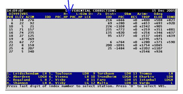
If interruptions in the Correction signal occur, this will have the consequence that the HP solution will not be calculated. Possibly the solution falls back to its' backup position, if so configured in the SPM menu. A possible cause can be grounding problems in the antenna cable.
