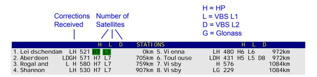
XP Corrections are not per reference station but for satellites, thus are not shown in the diagram above.
