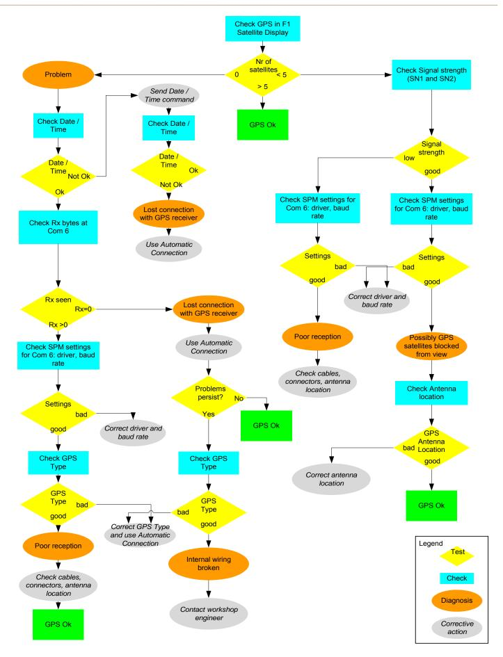
Figure 10 Trouble shooting GPS failure
