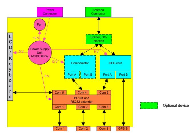
Figure 3 Internal Block diagram for HP Mobiles with internal demodulator (Topcon or LCE3000)
