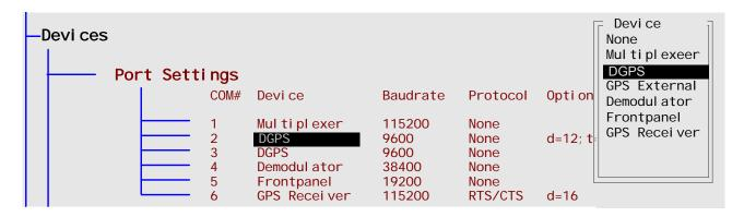
This menu is the extended menu from the menu Devices -> Port Configuration. The extension is protected by the Advanced menu and they can severely disable the HP Mobile from functioning. For example by removing the GPS Receiver driver one would break make the GPS Receiver non-detectable for the SPM software and hence no positions can be calculated.
