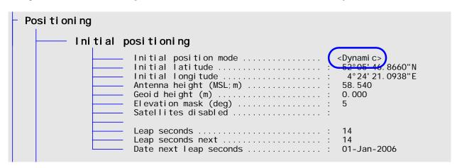
This Initial Position will then be used to seed the HP, XP and VBS positions. The user will also use this Initial Position to update the distances in the list of Reference Stations, as described a bit further down in 6.4.3.
