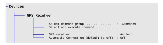
In this menu one is able to configure the internal GPS card directly. This is done by sending commands. It should be done with caution as one can alter the GPS in such a way that the SPM software is not able to use the data anymore. Or worse: is not able to communicate with the GPS anymore.
