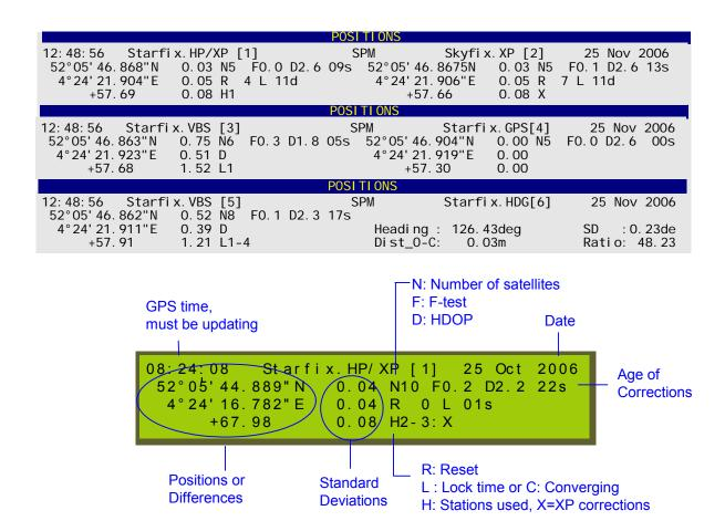
The Positions displays show the solution of HP, XP, VBS, GPS and HDG (Heading).
