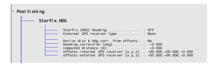
This Heading solution requires an External GPS receiver to be connected. In SPM Menu  $\rightarrow$  Devices  $\rightarrow$  Port Configuration (9.4.1) one should have the driver for External GPS Receiver selected and interface the GPS Receiver. Three types of GPS Receivers are supported: AshtechZ12, Topcon and Novatel. The HDG solution requires L1 and L2 for optimum performance. The GPS Receivers must be configured to output raw data.
