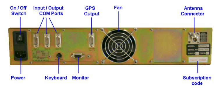
Connect serial cable to Com 2 or Com 3 to get HP Position as NMEA or HP\_MONITOR format. See further in manual on instructions for SPM software configuration.
