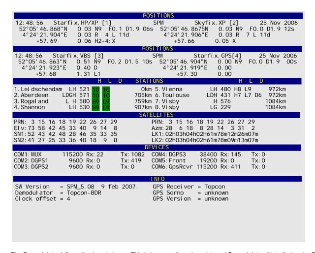
The Demodulator information is not shown. This is because there is no internal Demodulator. Note that under Devices none of the drivers is Demodulator either.
