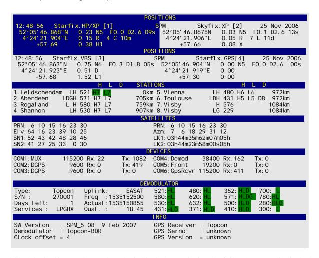
HP solution is still converging, as shown by the blue background colour, the C 10m (Convergencing for the last 10 minutes), and the Standard Deviations (SD Easting: 0.23 meter, SD Northing 0.15 meter and SD Height 0.38 meter).
