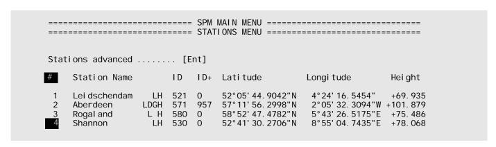
The length of the Station list can be expanded and reduced. This is explained in section 7.5 Expanding the list of Stations or Position Outputs. The maximum length of the list is 16 stations.
