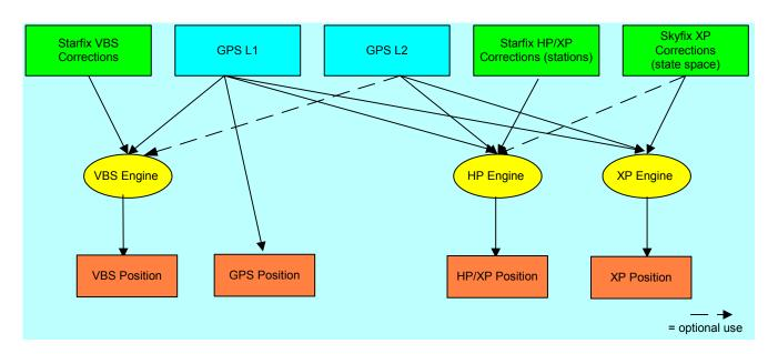
Figure 1 Four position solutions from SPM
