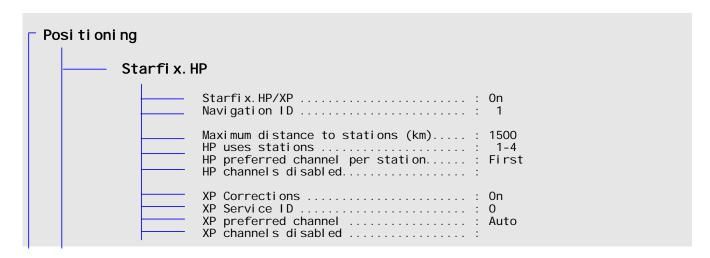
This menu contains the settings for the Starfix.HP/XP position calculation. The HP/XP position calculation can be configured such that it is Starfix.HP only, Starfix.XP only or a combined Starfix.HP/XP solution. Manipulate the menu items 'HP uses stations' and 'XP Corrections'.
