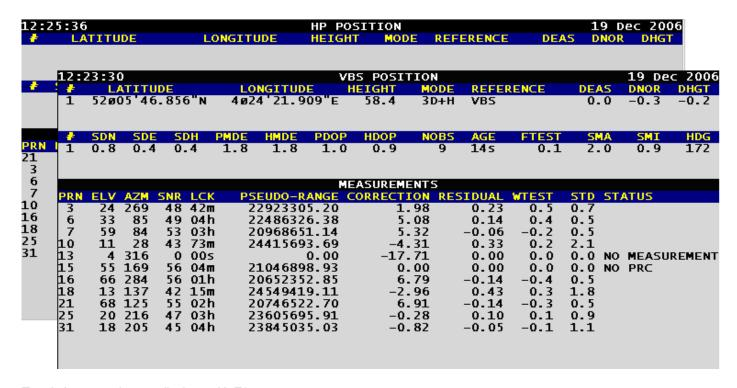
Toggle between the two displays with F3.
