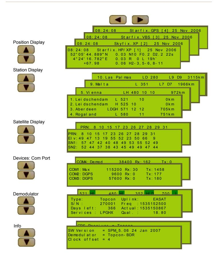
Figure 6: System Display - front panel
