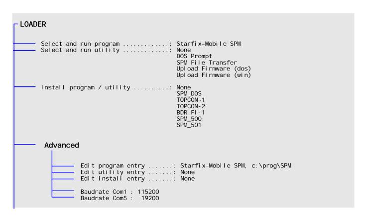
Figure 11: Loader Menu Structure
