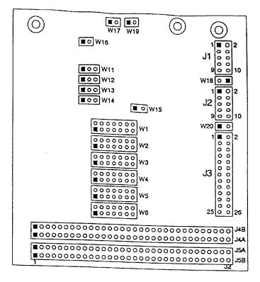
Figure 2-1. Connector and Jumper Locations
