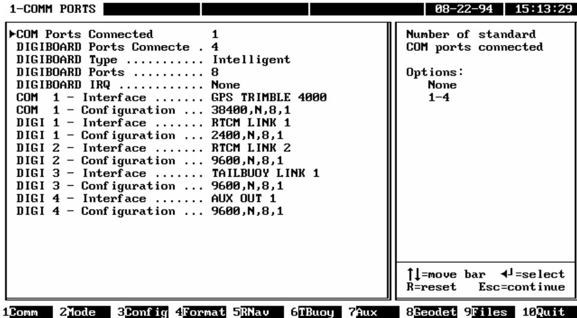
Figure 5.1: Communication set-up
