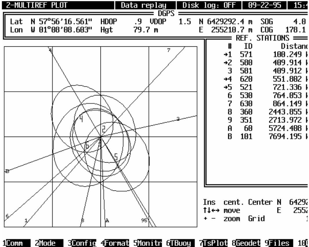
Figure 4.10: Reference station error ellipses and location-2
