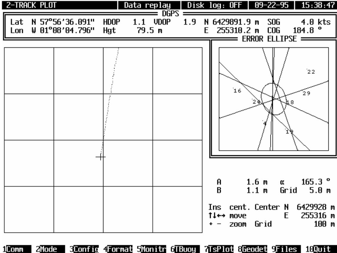
Figure 4.8: Track plot and error ellipse
