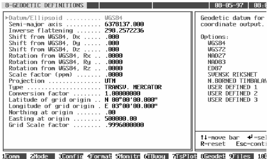
Figure 5.9 Datum and projection conversion factors
