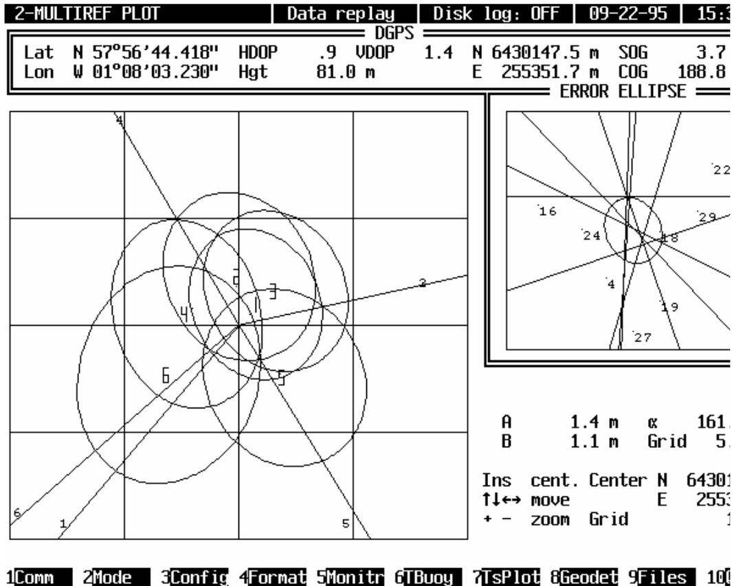
Figure 4.9: Reference station error ellipses and location-1
