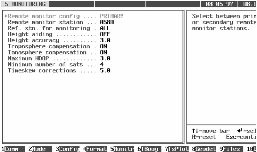
Figure 5.6: Virtual monitoring configuration menu
