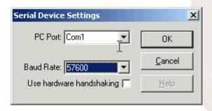
Confirm with <**OK**> twice. This will bring you back in the 'Open Configuration' window. Select <**Open**> GPSolution will now attempt to establish communication with the NovAtel OEM4 card
