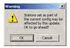
Changes such as the addition or deletion of beams and stations caused by reading a new .**SFX** will be reflected when configuring the <u>Starfix Decoder</u>. Any stations that had been used in calculations that were not present in the selected .**SFX** file will now be removed.
