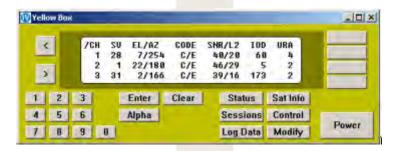
The *UTC* time displayed in the "Yellow Box" window will always be 1 or 2 seconds behind the UTC time shown in the Clock window. This is not a cause for concern as it is due to the time taken for the receiver to provide the front panel text.
