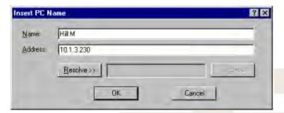
If the IP address is not known but the computer's network identification name is, and if all computers involved are aware of local naming services (WINS / DNS), then type in the computer's name in the "Address:" slot and click [Resolve>>]. Once the computer is found, its IP address will appear as shown. If required, use [>>Literal] to transfer the name and address to their named slots. Click [OK].
