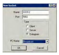
To target one specific PC requires that the Internet address of that PC should already have been identified. Explanation of adding PCs.
