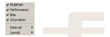
The averaging time used for the display can be set to 1 minute, 2 minutes or 5 minutes. (This does not change the Time Constant of the Filter itself). The averaging time is a moving window, losing the oldest adding the newest.
