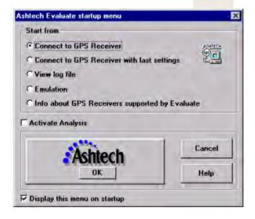
After installing the Evaluate software start the program by clicking the Ashtech Evaluate icon in the start menu. The user will be asked to choose a start up option. Select "Connect to *GPS* Receiver" and click [OK].
