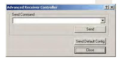
Select **[Send Default Config]** to complete the receiver configuration. Alternatively, type in known commands and select **[Send]** to send these to the receiver.
