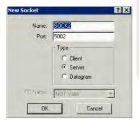
If the MultiFix computer is to be a server then there is no need to add the MultiFix computer to the PC table; the program already knows the computer's IP address. This can be seen in the window called up by "View" \ "Sockets".
