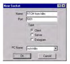
Enter the number of the port on which the Server PC is presenting the data. Change the socket's default name if required, current address.
