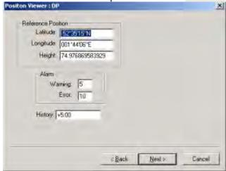
Set the alarm thresholds in metres and the "History", which is the period over which the stability will be determined. (see Position Viewer manual for more details).
