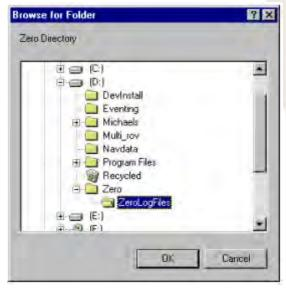
Be aware that typing in a non-existent path **will not create a folder**. If a new folder is required for data logging it must be created on the desired hard drive with Windows Explorer before logging begins. If a viable destination is not entered the \*.zer log files will be written into the MultiFix installation directory.
