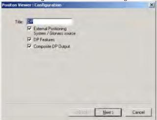
The wizard operates as a series of dialogues. Note that if at anytime an incorrect selection has been made, use [<Back] to retrace the steps through the wizard and make the correction.
