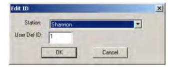
The "Edit ID" dialogue will appear. Make the necessary changes and click **[OK]** when completed. From the "Edit P2/94 Output" dialogue click **[OK]** to activate the output and complete the set-up. By clicking **[Cancel]** any changes will not be saved.
