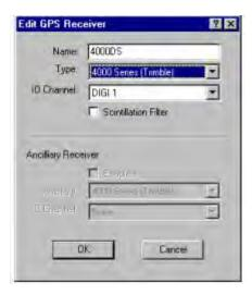
Enter a receiver name in the **Name** box. If this is left blank MultiFix will automatically assign a suitable name (e.g. 4000 DS (Trimble)). As with other name labels the program does not use it for receiver recognition purposes.
