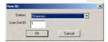
Select a station and then in the "User Def ID" enter a unique ID number to a maximum of 99 (MultiFix will not allow duplicate ID's). The ID does not have to represent the Starfix ID, but is used to identify the individual reference stations in the P2/94 T65 records. Once completed select **[OK]**. This process has to be repeated for each reference station that is to be included in the P2/94 output.
