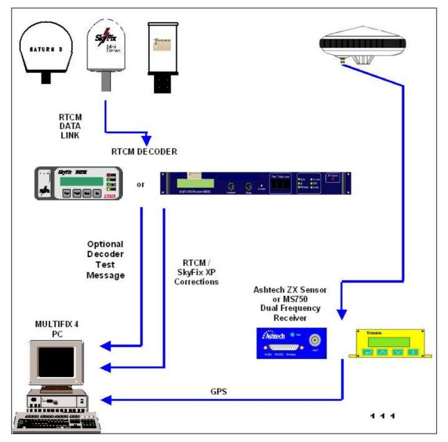
Figure 3. Example Interconnection with Ashtech ZX Sensor or Trimble MS750 Receiver
