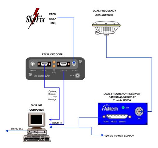
Figure 8 Example Configuration for SkyLink Options 3 and 4
