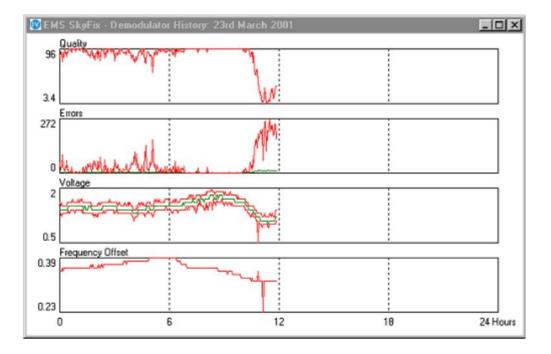
The Demodulator History display, found under "View" \ "Corrections" \ "SkyFix Decoder" \ "History" provides an illustrative summary of the stability of the SkyFix signal as recorded by the decoder. During scintillation on may see that the "Quality" drops, that the "Errors" increase and that the Minimum and Maximum "Voltage" separation widens.
