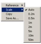
The scale of the display can be set to be 0.2, 0.5, 1, 2, 5, 10, or 50 metres from the centre to each edge. Alternatively it can be set to "Auto" in which case it will re-scale as required to show all the calculated positions and the error ellipses around those positions.
