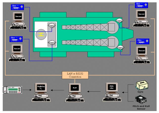
Figure 13 Example Interconnection with four GPS Receivers and soccer software
