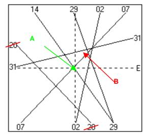
During periods of high ionospheric activity this cocked hat will be large (the solution will be divergent) due to ionospheric delay, the effects will therefore be greater. This effect will be reduced if dual frequency observations are used, as the cocked hat will once again be small.
