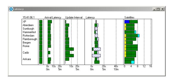
The example above has two rows of information for each dual frequency reference station. The first row refers to Type 1 messages and the second row refers to Type 15 or 55 messages where applicable. These will only appear once messages have been received. The Type 1 rows and Type 15/55 rows have different time scales as can be seen at the bottom of the Latency columns.
