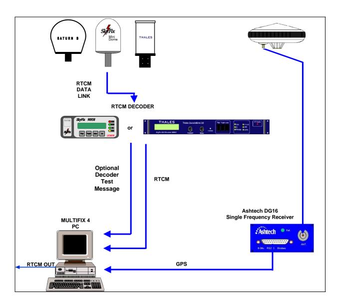
Figure 9 Example Configuration for SkyLink Option 5
