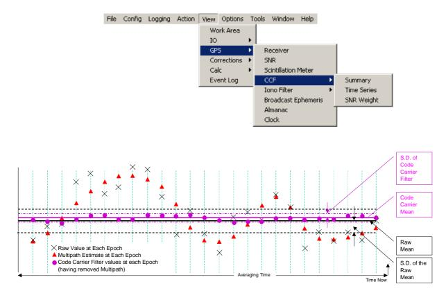
Figure 6 Graphical Representation of the Code Carrier Filter
