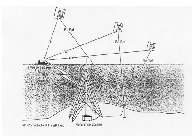
Figure 1.2 Differential GPS Concept
