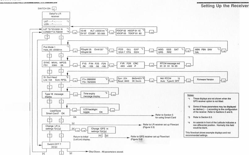
STM 1315 DeltaFix LR Receiver Type 90710 Operators Manual Pressing the  $\downarrow$  key will step through successive display pages to monitor current parameters in use and see the status of the unit in operation. The T key will step back through the displays; it will also allow the operator to go directly from the initial display to the Switch Off option.
