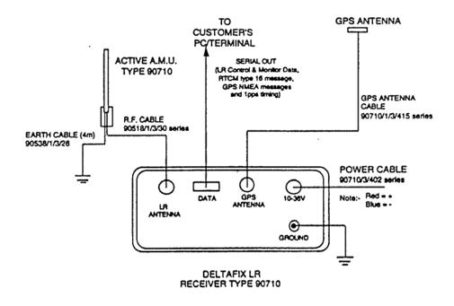
Figure 2.2 Receiving Station Equipment Interconnections (integral GPS receiver option)
