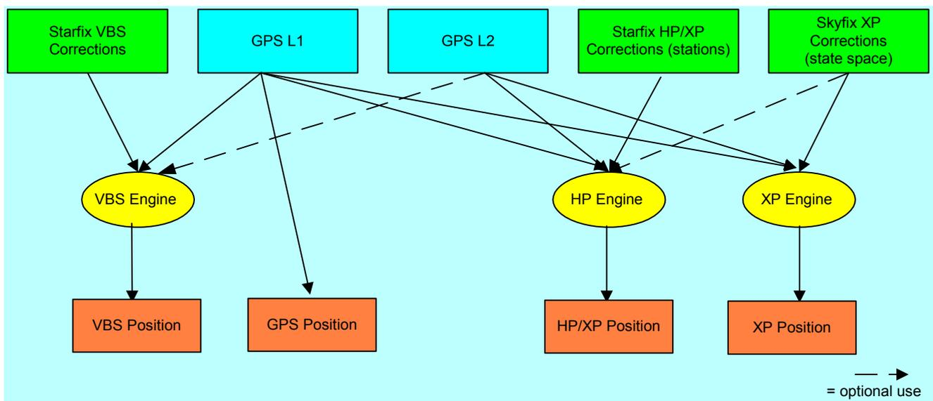
**Figure 1 Four position solutions from SPM**
