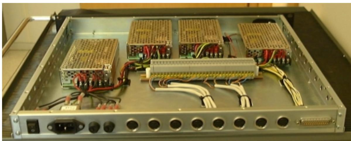
Figure 15 Rear of the Seatrack Junction Box
