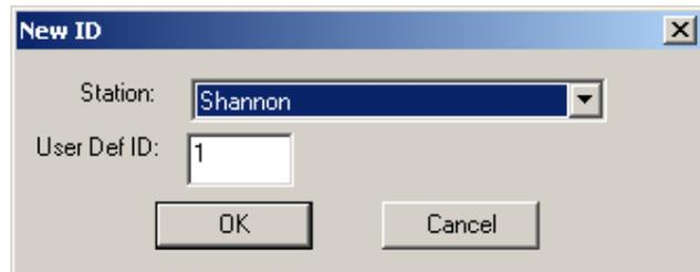
Select a station and then in the "User Def ID" enter a unique ID number to a maximum of 99 (MultiFix will not allow duplicate ID's). The ID does not have to represent the SkyFix ID, but is used to identify the individual reference stations in the P2/94 T65 records. Once completed select **[OK]**. This process has to be repeated for each reference station that is to be included in the P2/94 output.
