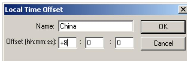
These can be used to provide a local time offset from UTC for the work area.
