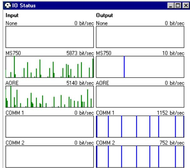
(When setting up Input / Output channels there is the option to select a dummy channel “None”. If selected the blue vertical bars would be seen progressing across the None Output box.)
