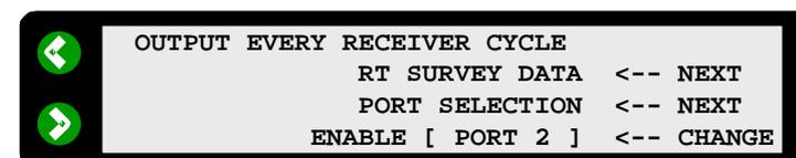
Ensure there are no other Receiver Cycle Outputs are enabled (Use Top ←Next)
