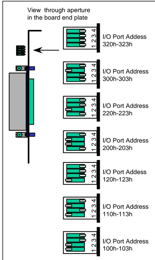
**Figure 1 PC/8e Switch Settings for IO Base Address**
