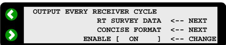
**Select the Port for the Receiver's Input of RTCM Corrections**
