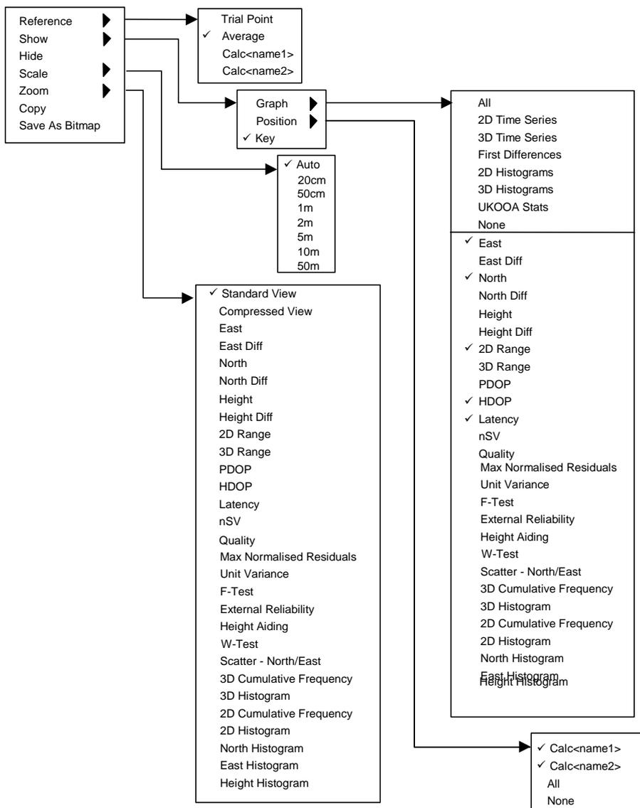
“Reference” allows the origin of the graphs displayed in the window to be changed.
