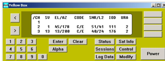
The UTC time displayed in the “Yellow Box” window will always be 1 or 2 seconds behind the UTC time shown in the Clock window. This is not a cause for concern as it is due to the time taken for the receiver to provide the front panel text.
