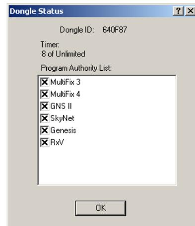
If the time limit of the dongle expires the program shuts down and an expiry message is posted.
