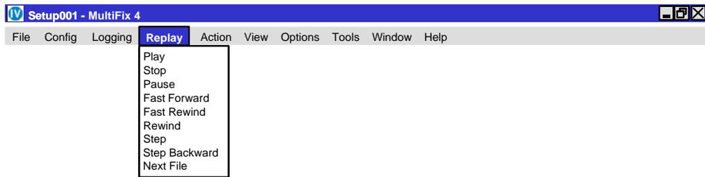
When Raw Zero files have been logged it is possible to re-inject that same information into MultiFix 4 by using the Replay option. Replay will read the Zero Log (\*.zer) files recorded by MultiFix 4 and create outputs, which MultiFix 4 can accept as source data. In Replay mode MultiFix 4 performs re-computations in pseudo-real time. See Section 4.3.4.1 on Zero logging on page 79.
