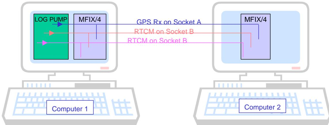
Figure 18 Example Configuration for Re-computation of Position Solutions
