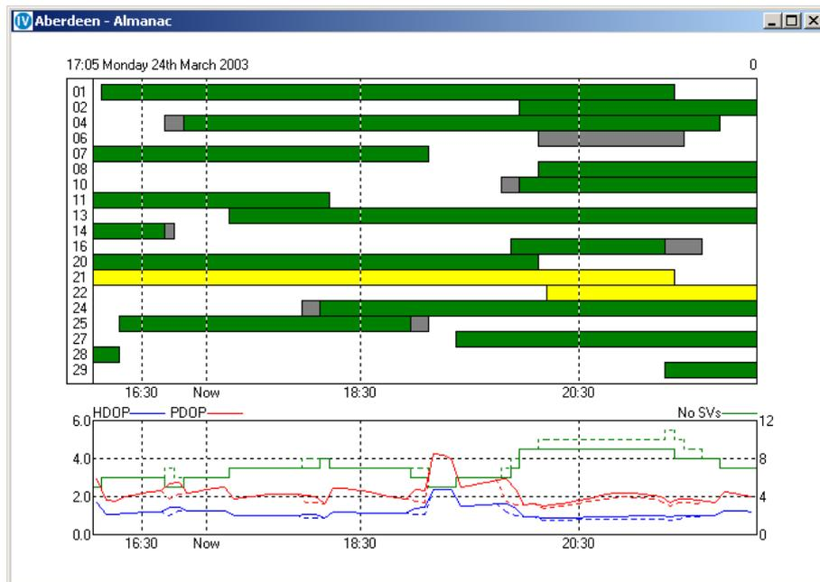
The top section of the Almanac window is a bar graph display of the availability of satellites over the previous 2 hours and the next 4 hours. This can be changed to a 24 hour view using the right click menu. The 24 hour view shows the current day, from midnight to midnight UTC.
