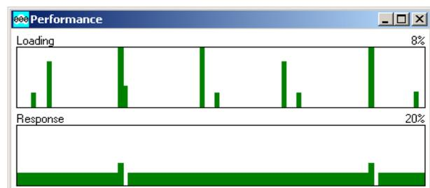
It is important there is enough time for all the processes to be completed in an orderly fashion. If there are too few resources the position solution may lag. The demand on the processor can be reduced by accessing only the data from the RTCM reference stations used in the computations, by having fewer computations and by closing windows.
