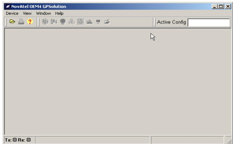
Create a “New...” configuration, for example with the name ‘OEM4’, or “Edit...” it to alter the settings.
