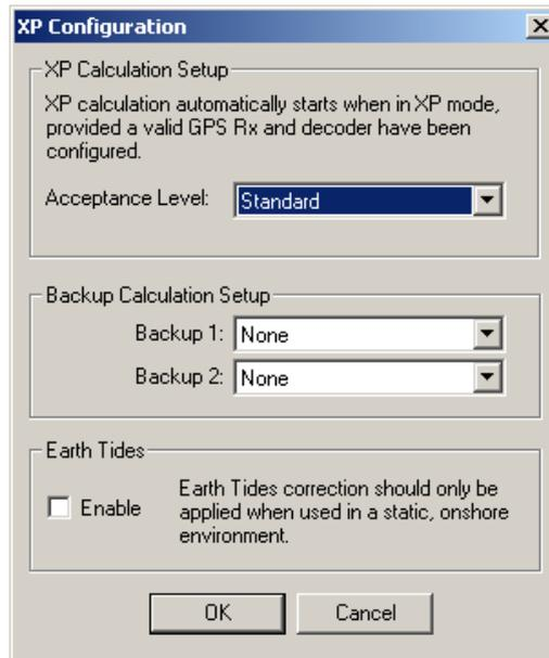
The “Acceptance Level” is used to set up how quickly XP solution will begin outputting a solution. There are four options:
