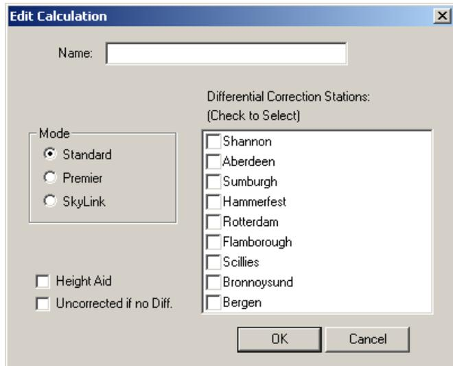
If SkyLink mode is selected all stations within a specified range threshold (the SkyLink Critical distance as defined in section 4.3.3.4.1) will be used. When a station lies outside of the range threshold it will only be used in dual frequency mode. Therefore, if a station only provides single frequency data and is outside of the critical distance it will not be used by MultiFix. If a station is within the range it will ONLY be used in single frequency mode.
