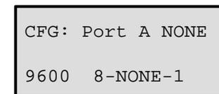
As it is assumed that SkyLink is connected to Port A, it is not necessary to configure ports B-1 and B-2. Toggle past these screens using the “v” button.
