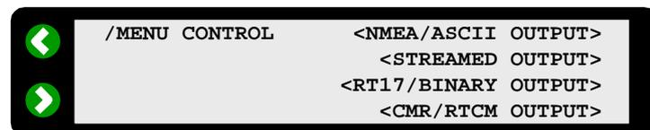
Using the “Enter” button to toggle to the desired parameter. Ensure that the correct output port is enabled and then set MEASUREMENTS and POSITIONS to 1HZ using the “Alpha” button. EPHEMERIS should be set to “ON” (optional) and all other parameters should be set to “OFF”.
