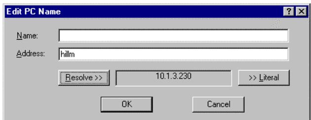
It is normal in a network for computers to be allocated new IP addresses when the PC is restarted. If the Client PC has a numerical entry for the address and the Server's address has changed, it will not be able to re-locate it. If the Client PC has the name of the Server PC in the address slot, it will automatically search to re-locate the Server PC by name. Assuming it is found, the Client PC will obtain the Server PC's current address.
