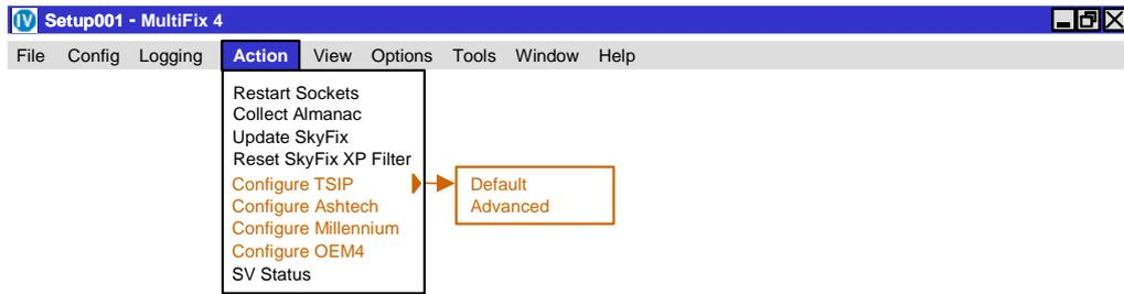
The Action menu item “Configure TSIP” will only appear if the GPS receiver selected uses the TSIP communication protocol, i.e. DSM (Trimble), BD112 (Trimble) or SK8 (Trimble).
