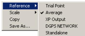
The first concerns the Origin to which the data is referenced point. It can be the Average of all the calculations, a static point, or any available computation.
