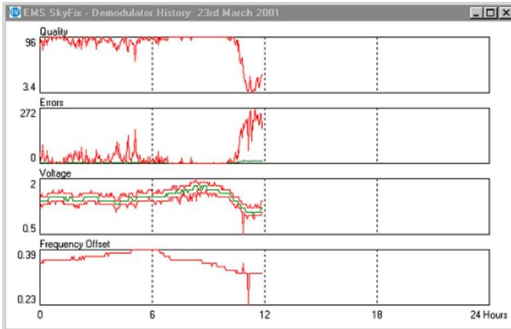
The Demodulator History display, found under "View" \ "Corrections" \ "SkyFix Decoder" \ "History" provides an illustrative summary of the stability of the SkyFix signal as recorded by the decoder. During scintillation one may see that the "Quality" drops, that the "Errors" increase and that the Minimum and Maximum "Voltage" separation widens.
