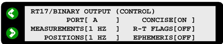
**The receiver must supply POSITIONS if SkyLink Option 4 or 5 Outputs are required.**
