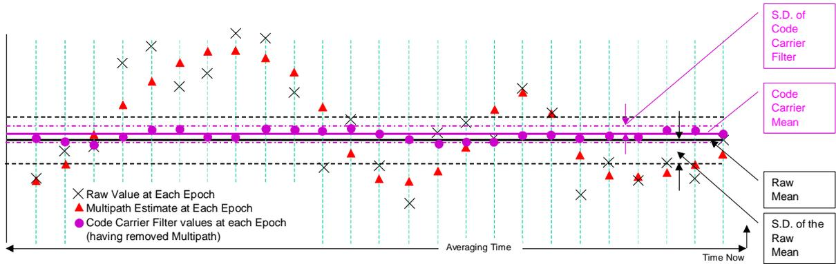
Figure 12 Graphical Representation of the Code Carrier Filter
