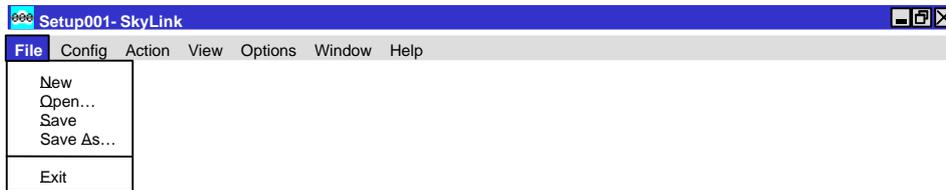
At the bottom of the “File” menu is a list of recently used configuration files. Clicking on one of these files opens up the chosen configuration.
