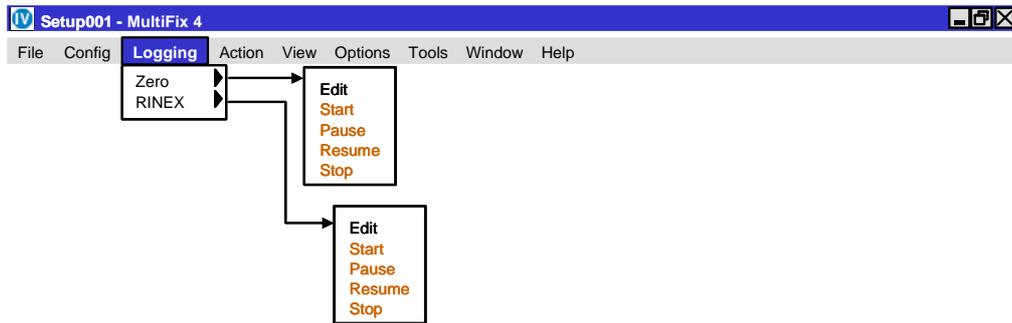
The Logging menu items shown above will change depending on the current state of logging. If no logging is taking place it will be “Edit” and “Start”, if logging is ongoing it will be “Pause” and “Stop” and if logging is paused it will be “Resume” and “Stop”.
