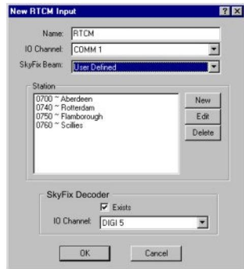
For Premier calculations there is no need to set up 6 reference stations if only one of them outputs Ionospheric error information as this will be the only station used in that mode.
