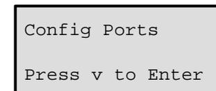
Press the “v” button to toggle to the Port A configuration display. Use the “>” button to enable and move the cursor and the “^” and “v” buttons to change the values, set the Baud rates to 9600, 8-None-1. Then press “↓”.
