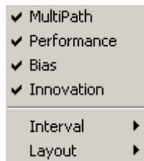
The averaging time used for the display can be set to 1 minute, 2 minutes or 5 minutes. (This does not change the Time Constant of the Filter itself). The averaging time is a moving window, losing the oldest adding the newest.
