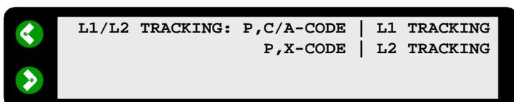
Only the L2 code can be disabled. Ensure that both the L1 and L2 codes are **enabled**.
