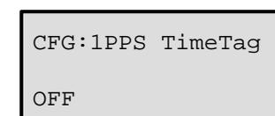
Toggle to the “Exit Config” display by pressing the “v” button. Press “↵” to exit this display. This completes the front panel configuration for the MS 750.
