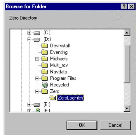
Be aware that typing in a non-existent path **will not create a folder**. If a new folder is required for data logging it must be created on the desired hard drive with Windows Explorer before logging begins. If a viable destination is not entered the \*.zer log files will be written into the Soccer installation directory.
