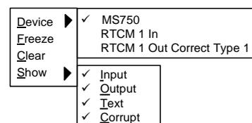
If “Device” is highlighted there is a sub-menu which lists the different input / outputs. Top of the list are the names given to the each of the GPS receivers. This is followed by the input from PDS.
