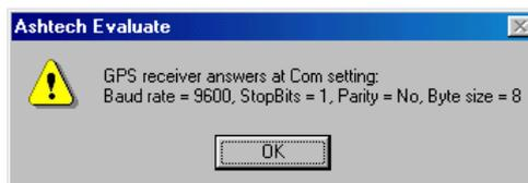
If no matching port settings are found, investigate all cable connections and make sure that the receiver is powered on.
