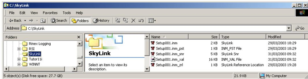
After installation and after a program run, SkyLink will have created / stored several files in the folder selected by the operator for the configuration file.
