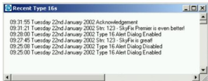
In addition, all received Type 16 messages are stored in a text file with a file name consisting of the configuration name and the days date (yyyymmdd), as below:
