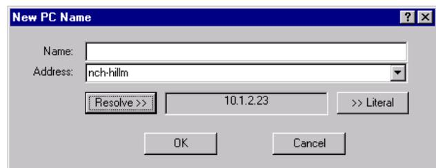
address and the Server's address has changed, it will not be able to re-locate it. If the Client PC has the name of the Server PC in the address slot, it will automatically search to re-locate the Server PC by name. Assuming it is found, the Client PC will obtain the Server PC's current address.
