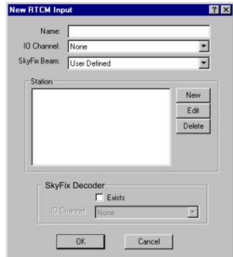
“SkyFix Beams:” contains a drop down list of all the satellite based Fugro RTCM sources. When one of those sources is selected, the dialogue is automatically populated with all the stations that carried by that system and the **[New]**, **[Edit]** and **[Delete]** buttons are lost.
