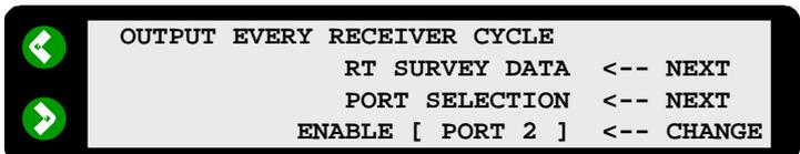
**Select the Format for the MultiFix 4/Trimble Receiver Communication**
