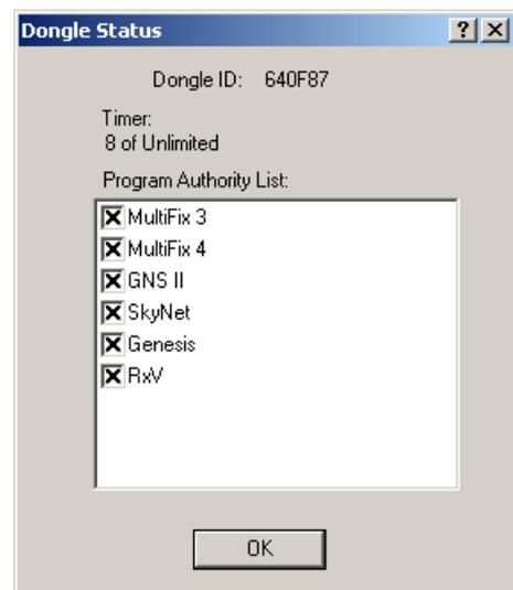
It is possible to revalidate the dongle by running the PROLIVE program and making a call to the Technical Support Group. The same program plus a telephone call can also be used to terminate a dongle so that it is no longer valid and no longer re-charged.
