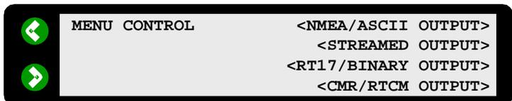
Using the **[Enter]** button to toggle to the desired parameter. Ensure that the correct output port is enabled and, using the **[Alpha]** button, set MEASUREMENTS and POSITIONS to 1HZ and CONCISE ON.
