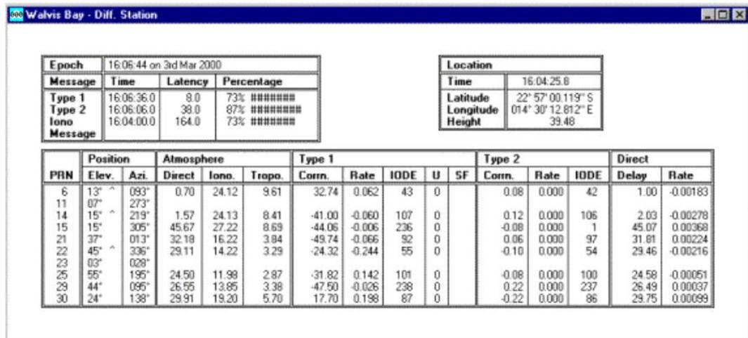
The window initially opens showing the first RTCM reference station. To have the window show data for another station, right click on the window and select the station.
