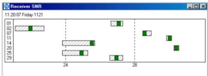
This second plot is taken from a period of scintillation and demonstrates the scale of the variation typically seen.
