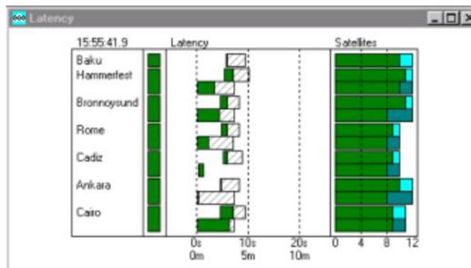
The example above has two rows of information for each dual frequency reference station. The first row refers to Type 1 messages and the second row refers to Type 15 or 55 messages where applicable. These will only appear once messages have been received. The Type 1 rows and Type 15/55 rows have different time scales as can be seen at the bottom of the Latency columns.
