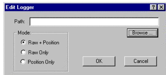
Select the folder into which the logged data is to go either by typing in the destination or by using the [Browse...] facility. This provides the Browse for Folder dialogue. The path can be defined by clicking on the desired destination folder.
