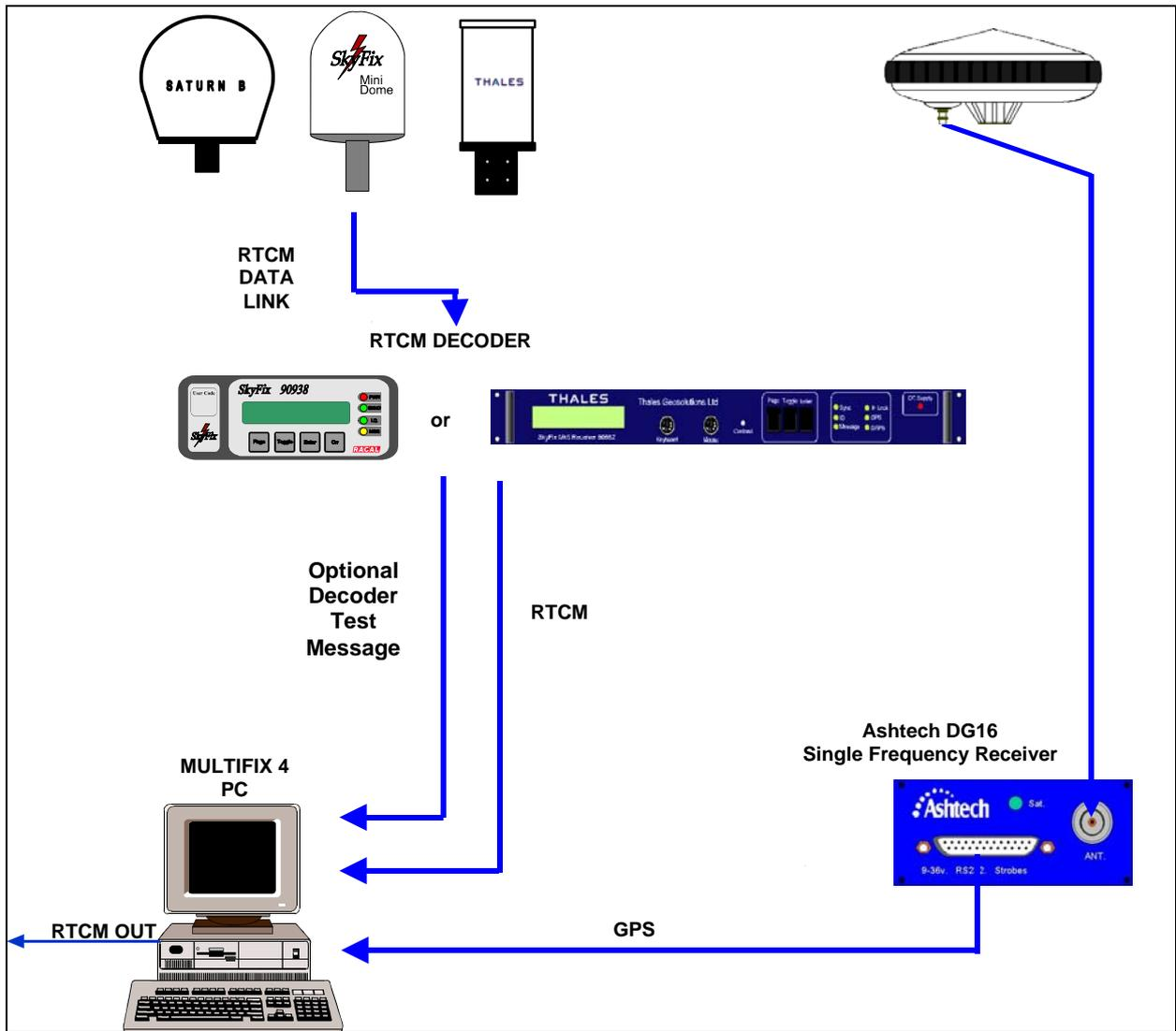
Figure 9 Example Configuration for SkyLink Option 5
