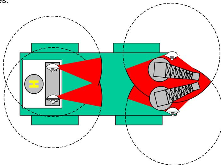
When the cranes are operational the masking situation changes. The cranes will be lifted from their normal location and rise far above the GPS antennas.
