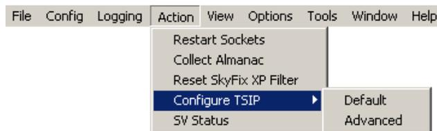
This facility instructs a Trimble Standard Interface Protocol (TSIP) GPS receiver to output the information MultiFix 4 requires. This will need to be done each time power to the receiver is cycled. (If a 90938 has a BD112 or DSM fitted there is battery back up on the receiver when the 90938 is switched off).
