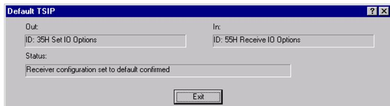
Synchronise Measurements message and an I/O Options message. As soon a response from the receiver is received the dialogue above will be shown. If there is no link between the computer and the receiver the dialogue will state “awaiting acknowledgement”, “unable to set default parameters” or “waiting to reset default receiver configuration”. Every 5 seconds it will retry to configure the receiver until **[Exit]** is clicked.
