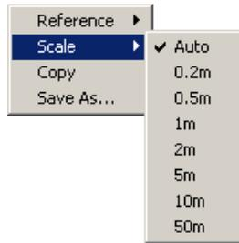
The scale of the display can be set to be 0.2, 0.5, 1, 2, 5, 10, or 50 metres from the centre to each edge. Alternatively it can be set to “Auto” in which case it will re-scale as required to show all the calculated positions and the error ellipses around those positions.
