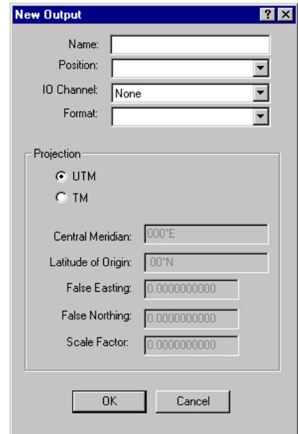
Grid co-ordinates will be based on the WGS 84 ellipsoid. There is no ellipsoid/datum transformation facility in MultiFix.
