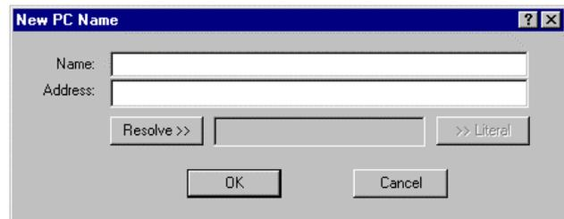
If the numerical IP address is known, enter a PC name in “Name:” and the IP address in “Address:” and click **[Resolve>>]**. Click **[OK]**.
