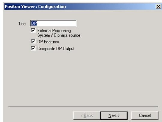
The "DP Features" option will enable the auto select mode for selecting the most stable solution.
