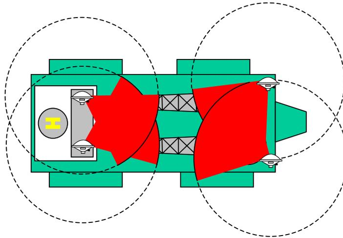
The two heavy lift cranes cause some obstruction, even when stowed. This can be in the form of direct blockage or as multipath and is marked in red on the diagram.
