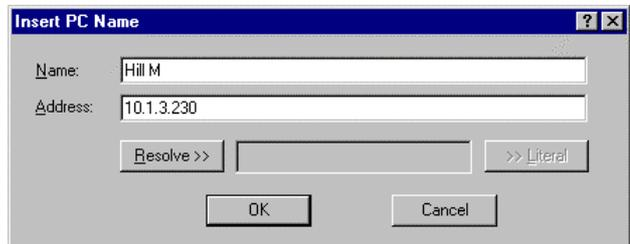
If the IP address is not known but the computer’s network identification name is, and if all computers involved are aware of local naming services (WINS / DNS), then type in the computer’s name in the “Address:” slot and click **[Resolve>>]**. Once the computer is found, its IP address will appear as shown. If required, use **[>>Literal]** to transfer the name and address to their named slots. Click **[OK]**.
