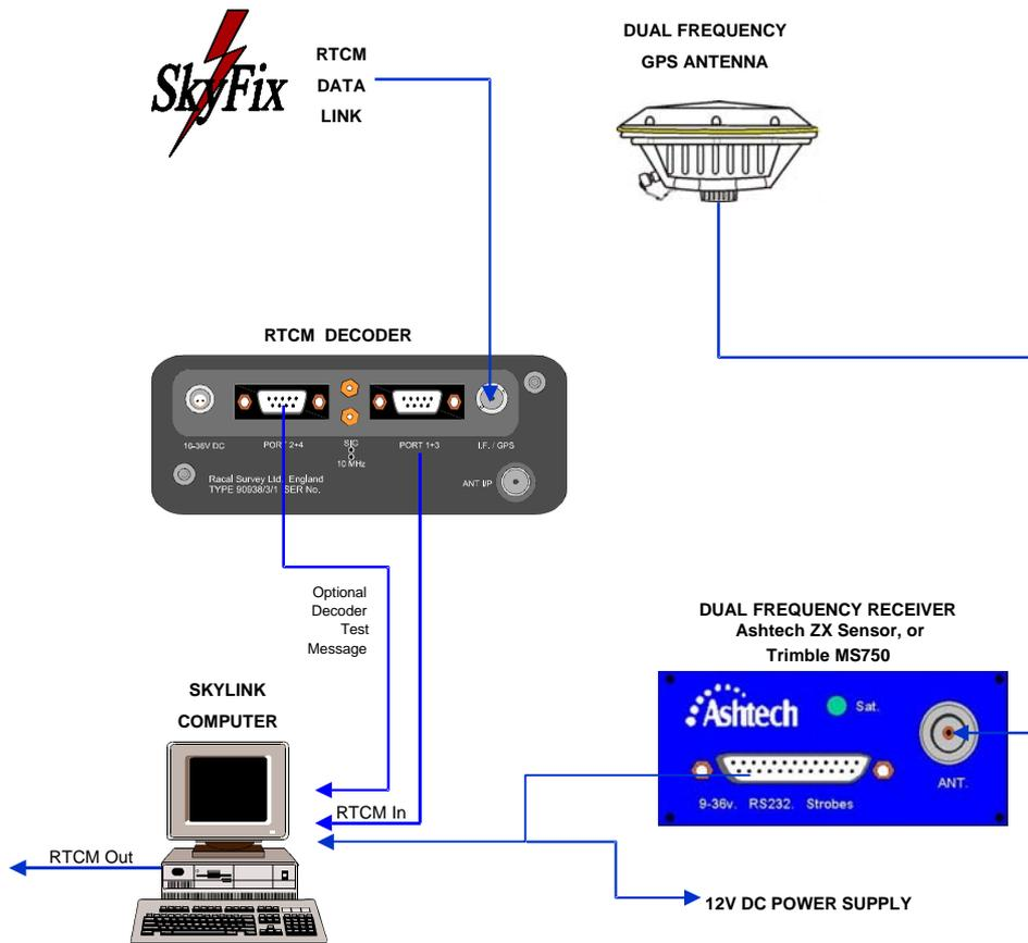
Figure 8 Example Configuration for SkyLink Options 3 and 4
