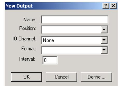
The “Interval” option allows the user to specify an interval (in seconds) between GGA outputs, to be used if an output rate of less than 1Hz is required.
