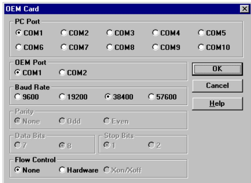
In case this procedure fails to establish a connection at a 57600 baud rate and establishes communication at a lower rate, the following steps allow the user to change the speed of the port.
