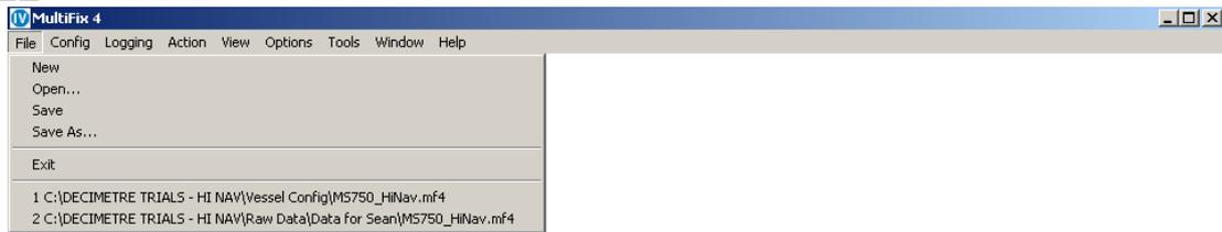
At the bottom of the “File” menu is a list of recently used configuration files. Clicking on one of these files opens up the chosen configuration.
