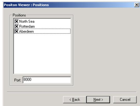
This will set up the required socket configurations in both MultiFix and Position Viewer. It will also create corresponding inputs and outputs in both applications. The ZeroLink data format is used so only one data port is required.
