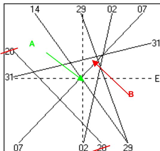
During periods of high ionospheric activity this cocked hat will be large (the solution will be divergent) due to ionospheric delay, the effects will therefore be greater. This effect will be reduced if dual frequency observations are used, as the cocked hat will once again be small.
