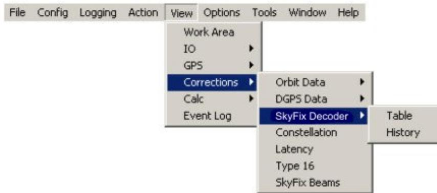
Assuming the SkyFix Decoder option has been enabled and given an IO channel, see Section 4.3.3.3.1 on page 60, the output from the decoder can be viewed.
