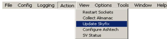
This function allows the user to update the SkyFix beams and station lists within MultiFix by means of an XML file with the extension \*.sfx without having to wait for a new software release. When changes are made to the SkyFix network a new XML file will be made available to MultiFix users allowing them to update their software.
