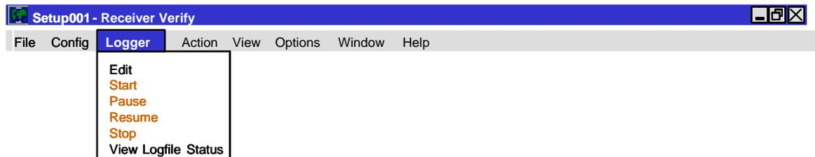
The Logger menu items shown above will change depending on the current state of logging. If no logging is taking place it will be "Edit" and "Start", if logging is ongoing it will be "Pause" and "Stop" and if logging is paused it will be "Resume" and "Stop".
