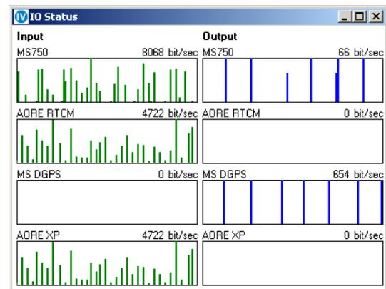
(When setting up Input / Output channels there is the option to select a dummy channel “None”. If selected the blue vertical bars would be seen progressing across the None Output box.)
