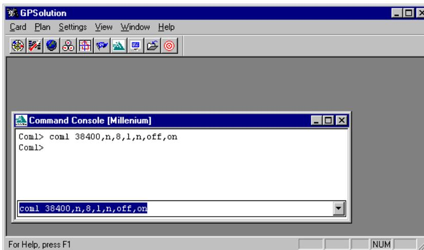
Upon changing the baud rate, you will lose communication with the card. In this case, close the GPSolution application and restart using the configuration file created earlier.
