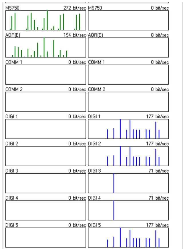
In the IO Status window the latest time is in the centre between the Input and Output columns. Each box indicates when data has been input or output, over the last 5 seconds, on that port by scrolling vertical bars from the centre to the outside edges of the window. The box re-scales such that the greatest data rate over the last 5 seconds is full scale. The current bit rate is shown opposite the I/O channel name.
