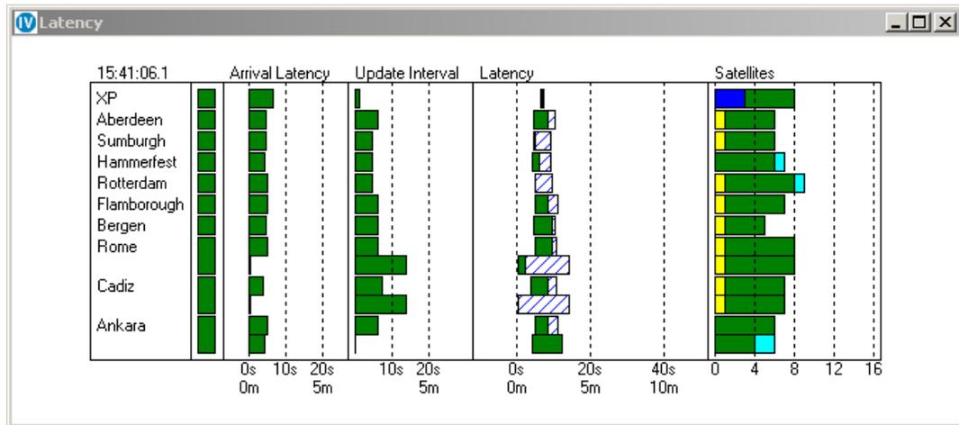
The example above has two rows of information for each dual frequency reference station. The first row refers to Type 1 messages and the second row refers to Type 15 or 55 messages where applicable. These will only appear once messages have been received. The Type 1 rows and Type 15/55 rows have different time scales as can be seen at the bottom of the Latency columns.
