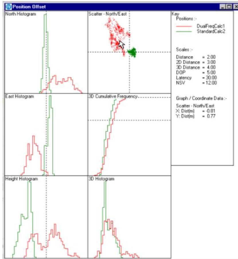
If a graph is to be viewed in more detail it can be selected individually in the Zoom selection menu. Any graph can be called up and it will fill the window, it does not need to be already open. To zoom into a graph that is already displayed double-click on the desired graph. To revert to the original display double-click on the graph again.
