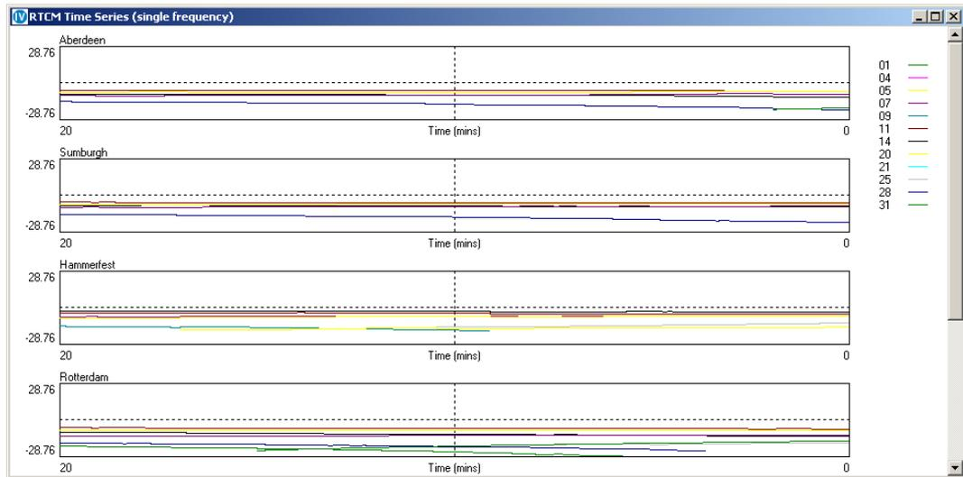
Right clicking on this window gives various options. Selecting a station in “Differences” will then difference all data to that station. This indicates how closely the positions for each satellite match at the selected reference stations.
