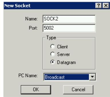
To target one specific PC requires that the Internet address of that PC should already have been identified. See Section 4.3.3.1.2.1 on page 55 for an explanation of adding PCs.
