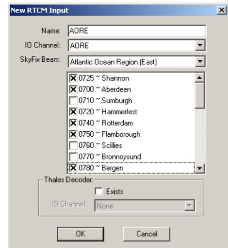
The program requires the station ID code number. A name is also required for identity purposes but is not significant in accessing the data.
