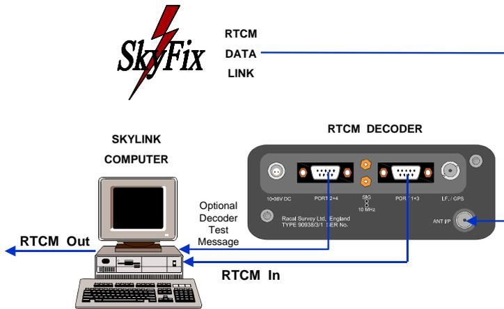
Figure 7 Example Configuration for SkyLink Options 1 or 2
