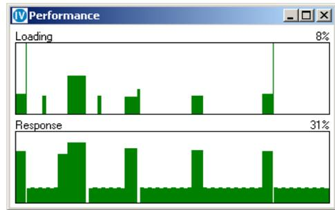
It is important there is enough time for all the processes to be completed in an orderly fashion. If there are too few resources the position solution may lag. The demand on the processor can be reduced by accessing only the data from the RTCM reference stations used in the computations, by having fewer computations and by closing windows.
