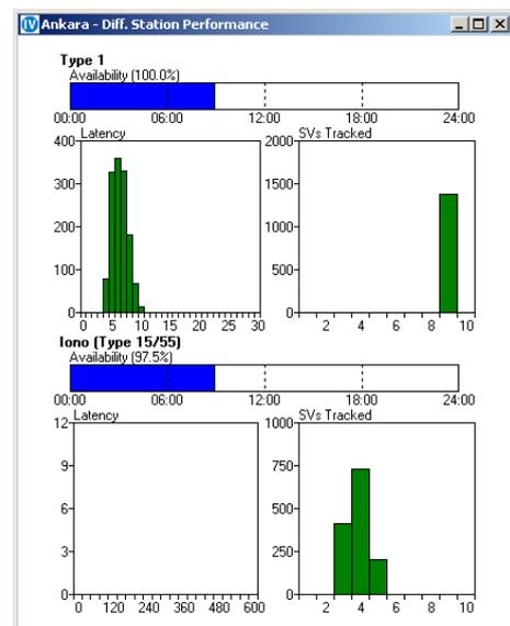
correction messages. If the reference station has not got the capability to transmit Type 15 or 55 messages then that part of the window remains blank.
