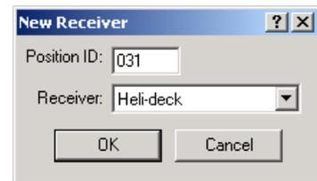
Each GPS receiver to be used in the calculation should be individually defined in this way. Settings can be changed at a later stage by using the “Edit..” button, or receivers deleted from the calculation using the “Delete..” button.
