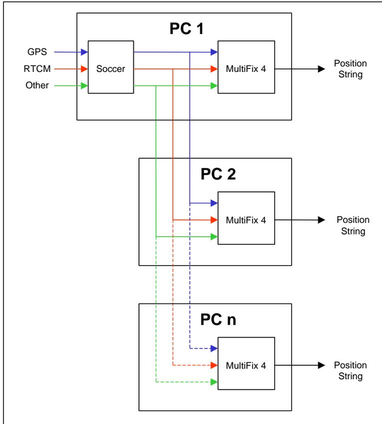
**Figure 17 Outputs Available from Soccer Configuration**
