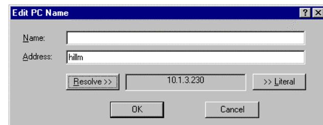
will not be able to re-locate it. If the Client PC has the name of the Server PC in the address slot, it will automatically search to re-locate the Server PC by name. Assuming it is found, the Client PC will obtain the Server PC's current address.
