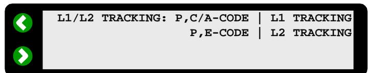
Only the L2 code can be disabled. Ensure that both the L1 and L2 codes are **enabled**. The diagram above shows the screen display for the 4000 SSI receiver in dual frequency mode. The display on the 4000 SSE receiver differs slightly: the **L2 TRACKING** codes will read **P,X** instead of **P,E**.
