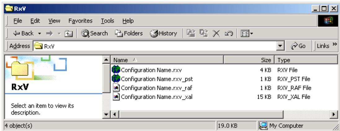
The \*.rxv is the core RxV configuration file and is stored in XML format.
