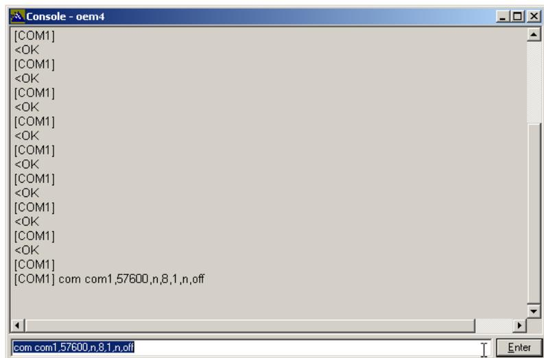
Upon changing the baud rate, you will lose communication with the card. In this case, close the GPSolution application and restart using the configuration file created earlier, but changing the baud rate to 57600 in 'Device Settings'.
