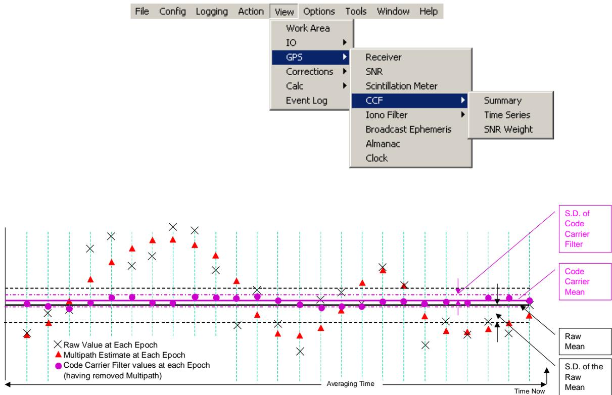
Figure 6 Graphical Representation of the Code Carrier Filter
