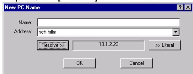
It is normal in a network for computers to be allocated new IP addresses when the PC is restarted. If the Client PC has a numerical entry for the address and the Server’s address has changed, it will not be able to re-locate it. If the Client PC has the name
