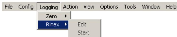
MultiFix 4 has the capability to log raw GPS observation in the RINEX (Receiver Independent Exchange) format. This is used to collect data for carrier phase post processing; typical usage is for verification after a final fix or for a post-processed RTK solution.
