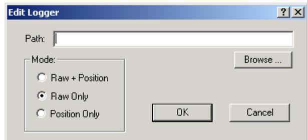
Select the type of logging required. Note there are not separate raw and position files, the Zero Log (\*.zer) files can contain both raw measurement and position data.
