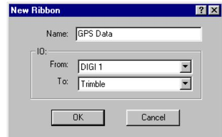
Select “Config” \ “Ribbon” \ “New...” and the New Ribbon window will appear. Give it a name and then select the relevant Input and Output location. To apply this ribbon click **[OK]**. From the “View” menu select “IO Status”. The **Output** column should show data being output from the program on the relevant port or socket.
