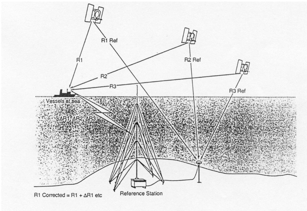
Figure 1.2 Differential GPS Concept
