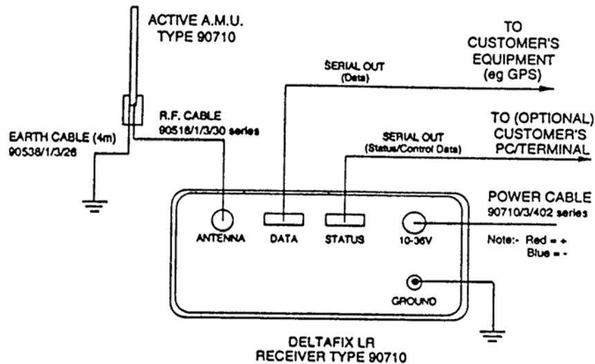
Figure 2.1 Receiving Station Equipment Interconnections (external GPS receiver option)
