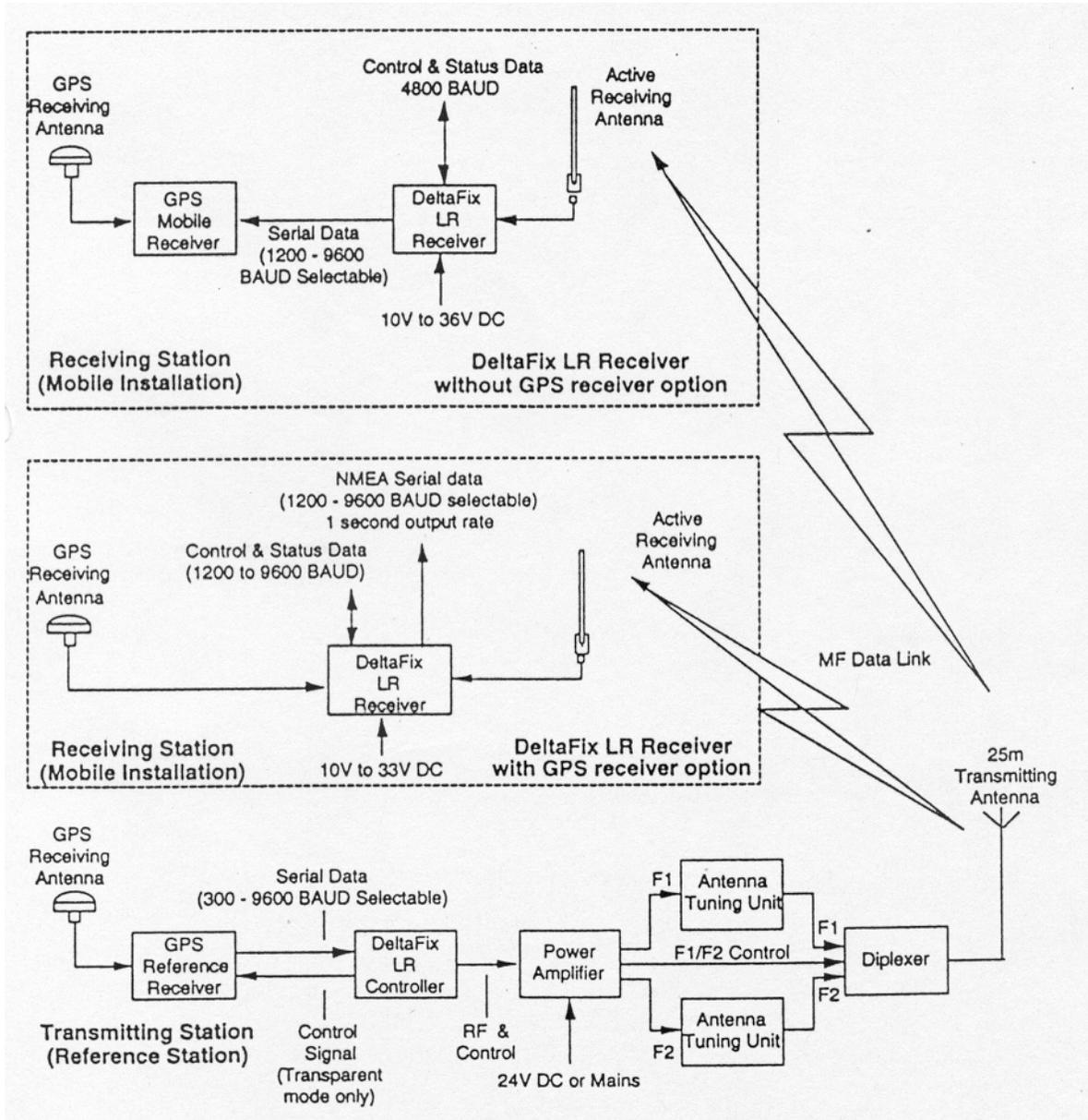
Figure 1.3 DeltaFix LR System Block Diagram
