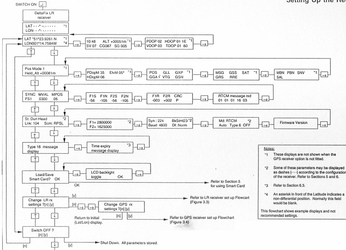
Pressing the ↓ key will step through successive display pages to monitor current parameters in use and see the status of the unit in operation. The T key will step back through the displays; it will also allow the operator to go directly from the initial display to the Switch Off option.
